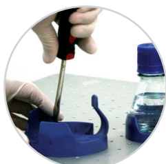
Screw clamp on shaker platform
